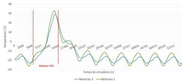
Fig. 16. Batteries temperatures without active thermal control
