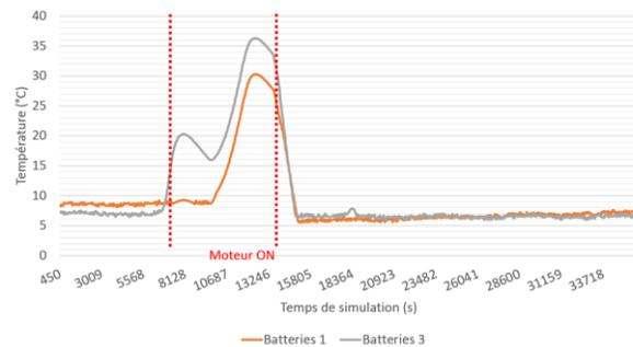
Fig. 17. Batteries temperatures with hot resistors
