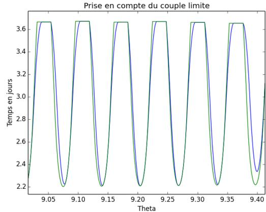
Fig. 5. Optimal and actual orientation of the satellite
