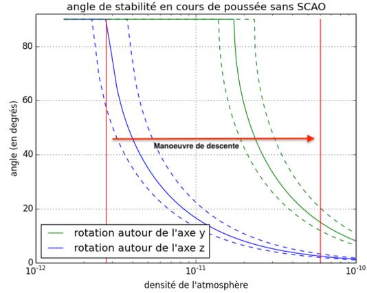
Fig. 10. Stability angle with respect to the atmosphere density
