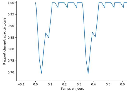
Fig. 8. Depth of discharge of the batteries over 2 cycles
