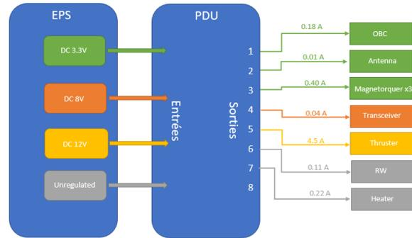
Fig. 9. Electric architecture
