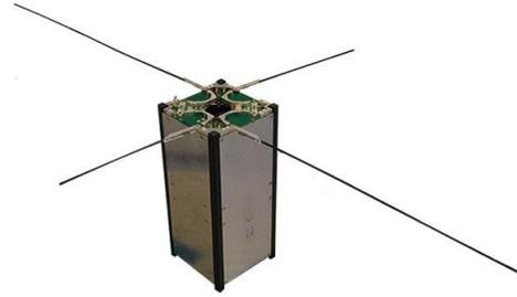
Fig. 12. Example of deployed UHF antennas
