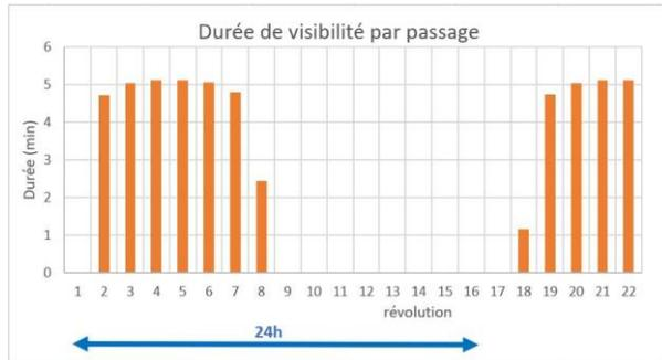
Fig. 11. Visible time over the ground station per orbit
