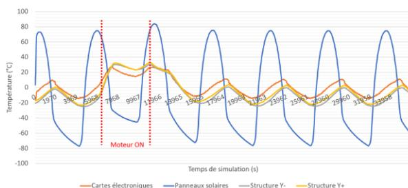
Fig. 15. Temperatures of the subsystems (electronics, structure in red and yellow; solar panels in blue) with radiative paint on the satellite
